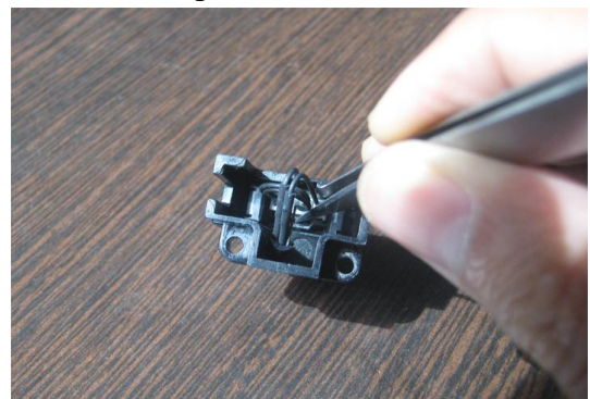
4.Use tweezer poke the inside clip then take the of the IC out
