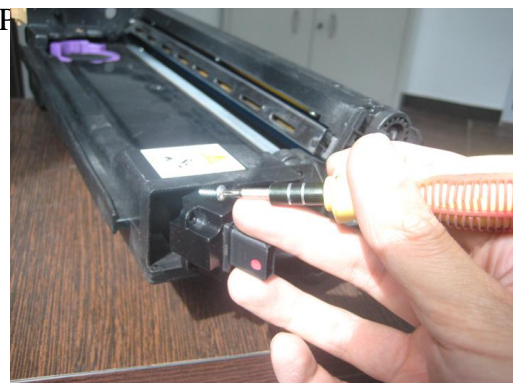
8.At last, put the intact seat into the toner cartridge.
